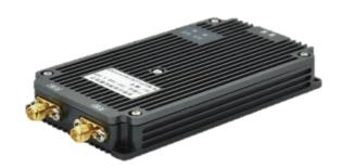
The airborne self-organizing network radio is mounted on the launch platform and achieves long-distance communication across regions through aerial multi-point relay and dynamic cluster networking. it can be mounted on various heterogeneous launch platforms, with low network latency and large scale, up to 256 nodes.
